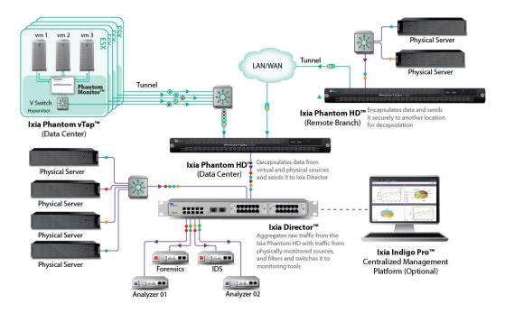
The Ixia Phantom HD turns virtual traffic into physical packets and works with Ixia's network access and management solutions. It aggregates traffic from remote facilities to your destination of choice.
