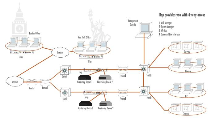
iTap Port Aggregators form an early warning system to detect network anomalies.
