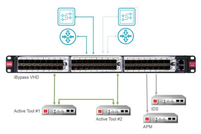
iBypass VHD flexibility example: with a failover network connection configured, iBypass VHD passes the traffic from a single network link to two serial inline tools and creates copies of the same traffic that is regenerated to two additional out-of-band tools.
